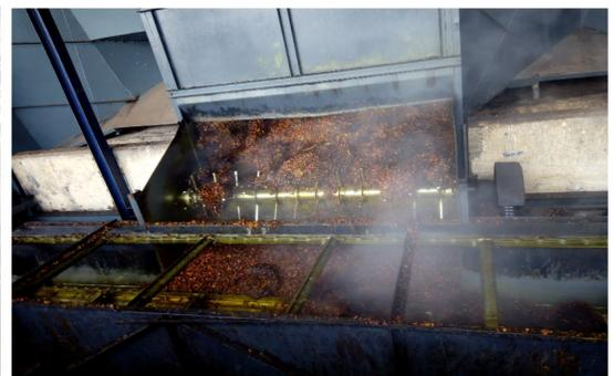
\*FFBs after cooking in the sterilizer been moved to the thresher for further processing.
