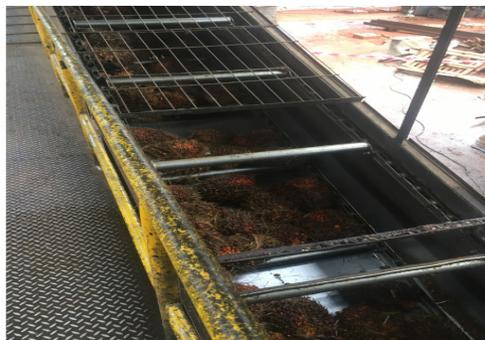
\*Fresh FFBs been moved from the conveyor to the sterilizer at the Okomu 1 Palm oil mill
