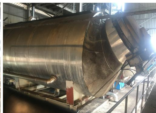
\*37-ton capacity tilting sterilizer for cooking FFBS, Presco
