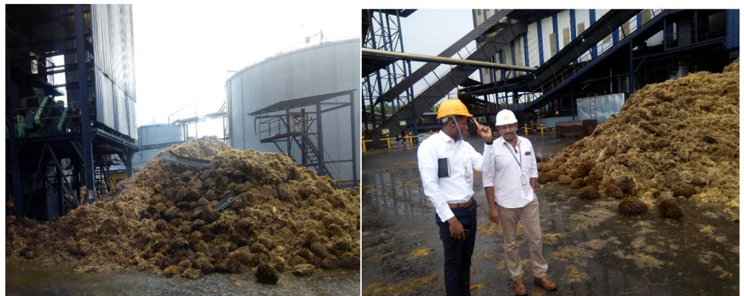
\*Raw material waste; Empty fruit bunches (EFBs) and fibre used in the fueling the Turbine
